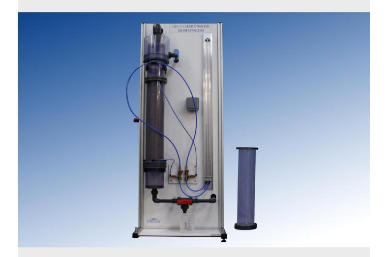
With the equipment HD 11.1, it is a question of knowing the ease that a land has, to the passage of the water inside, by obtaining its coefficient of permeability k, applying the Law of Darcy.
